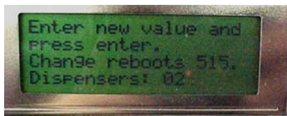
Mode 51 – Programming the number of Fueling Points
