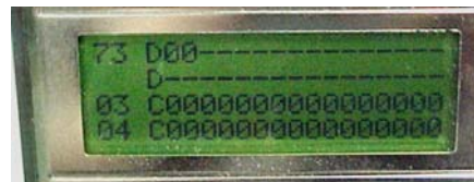
Mode 51 – Programming the number of Fueling Points
