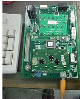
Figure 17.2 Backside of Local Preset Board With PC Keyboard connected
