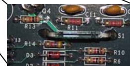
Reed Switch for gaining access to Totals.
